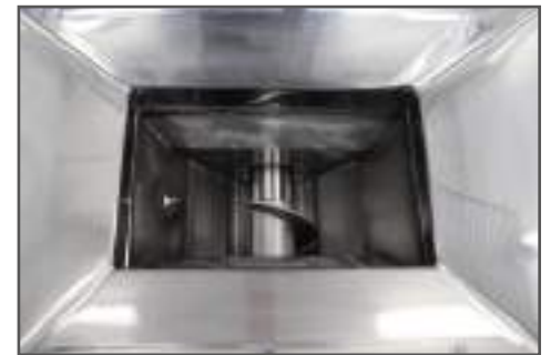
Top view of hopper infeed of scanEmul 175 – Hopper Fed.
