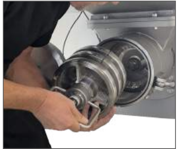
View of easy mounting of the knife cassette.
