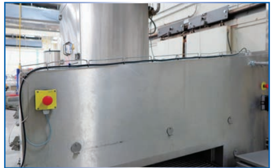
HYGIENICALLY DESIGNED SLOPED SURFACES FOR WATER RUNOFF
