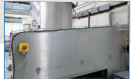
HYGIENICALLY DESIGNED SLOPED SURFACES FOR WATER RUNOFF
